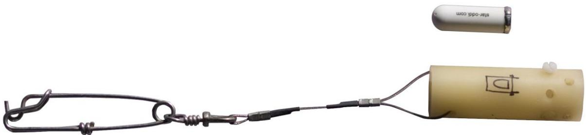
**Figure 2.** TDR and housing, total length including clip is 32cm
