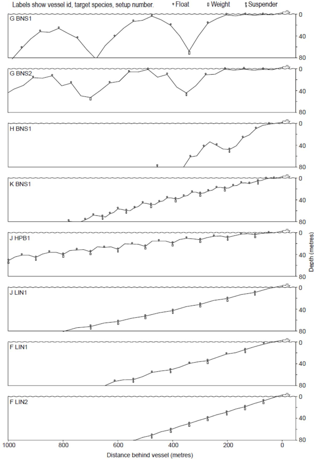
**Figure 8.** INTIAL RESULTS - composite profiles of longlines sinking behind vessels for the different line setups investigated. BNS denotes bluenose, HPB hapuku and LIN ling.
