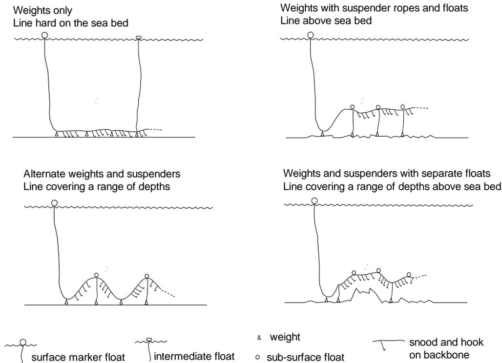
**Figure 1.** Example line configurations.
