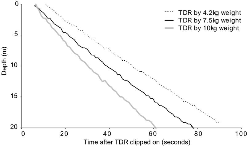
**Figure 3.** Time-depth profiles for TDRs on the same line positioned next to different sized weights
