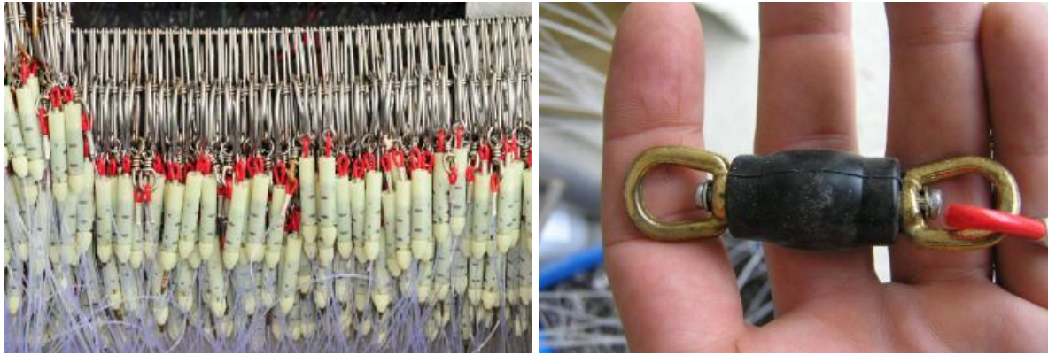
Figure 3. L: Luminous sliding leads stored onboard pelagic longline vessels. Hooks may be set with weights placed at variable distances from the hook (Photo: Fishtek Ltd). R: Weighted swivels are a conventional approach to branchline weighting in pelagic longline fisheries (Photo: https://www.afma.gov.au/environment-and-research/reducing-bycatch/bycatch-reduction-devices/line-weighting-pelagic/ ).
