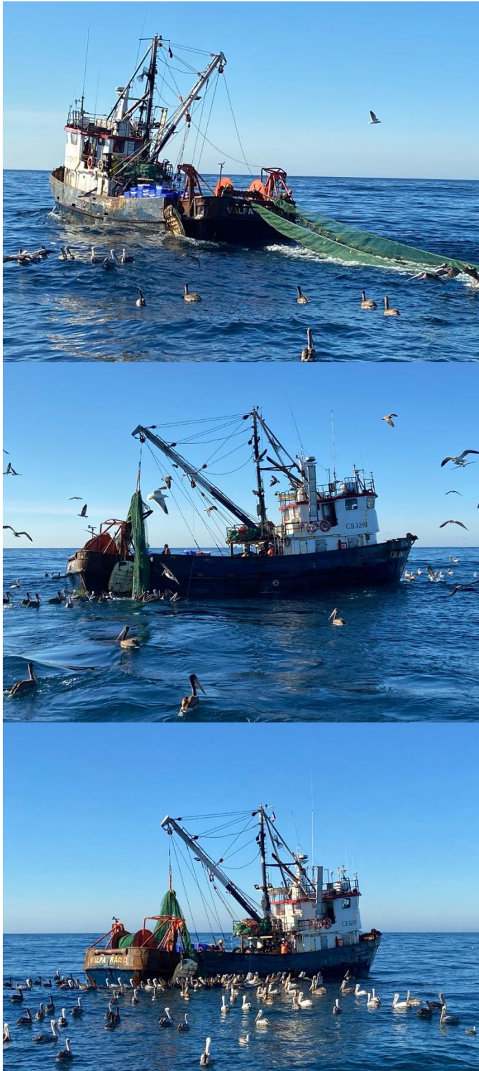
Figure 2. Side-haul process for small trawl vessels for crustaceans in the HCS, Chile. Note the pass of the cod-end over the stern arch of the starboard side.
