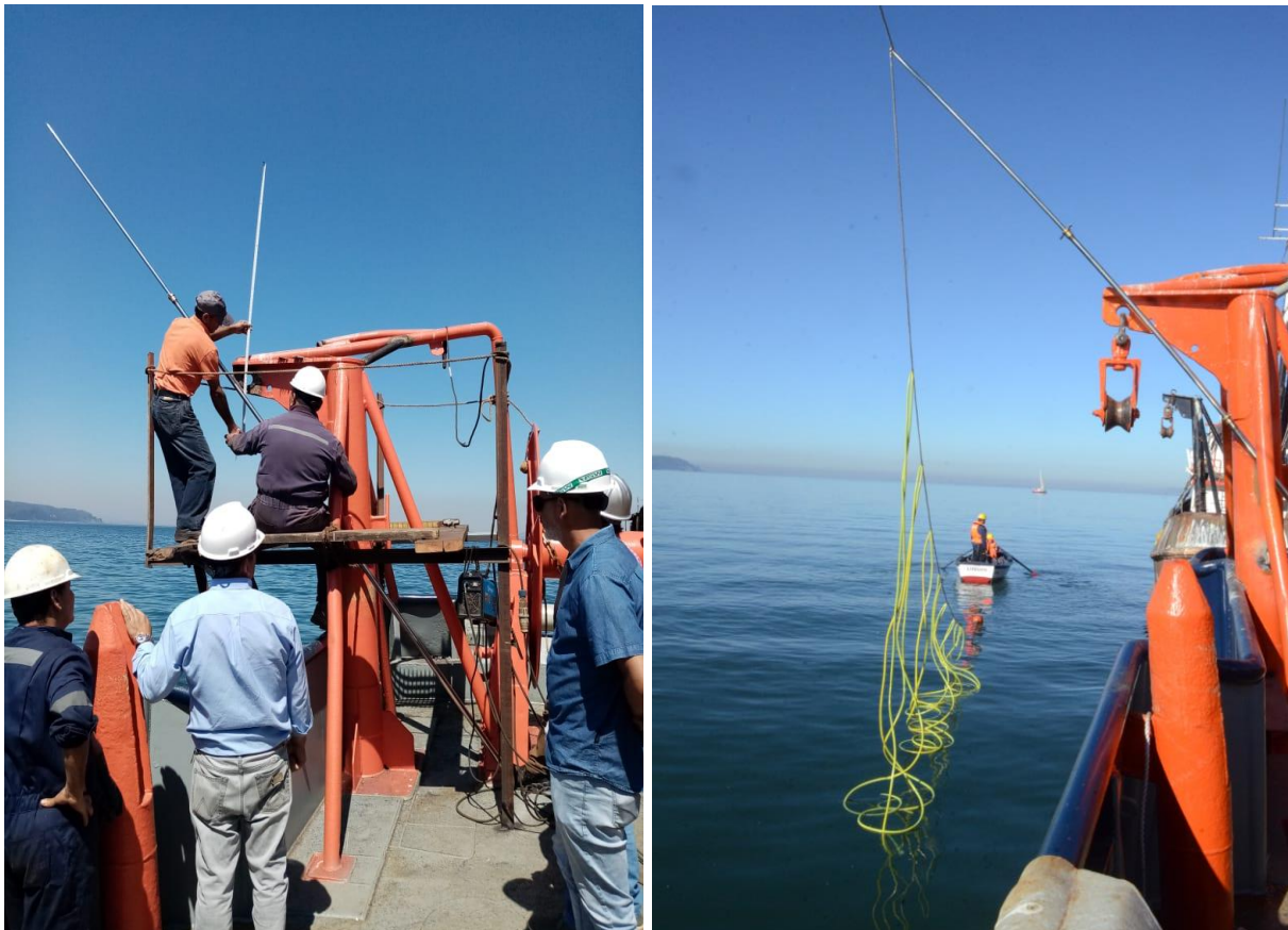
Figure 3. Extension arm prototype for side-haul small trawl vessels in the HCS, Chile.
