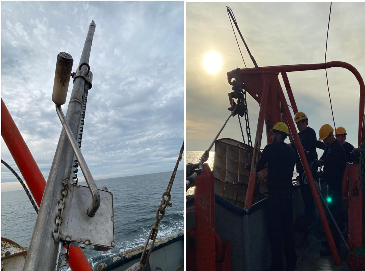
Figure 4. Extension arm with handle-crank system for small demersal trawl vessels in the HCS, south-central Chile.
