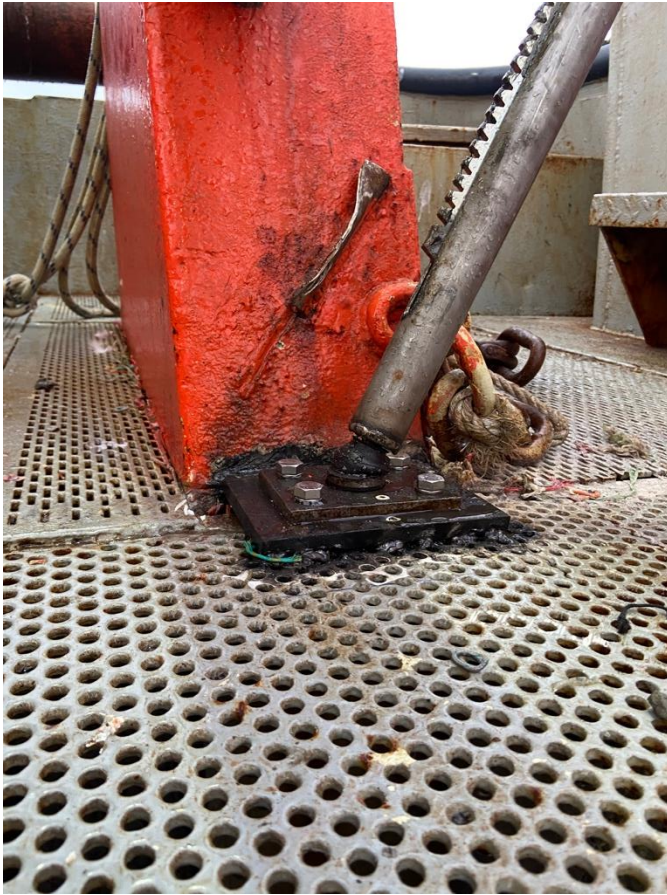
Figure 5. Base of the extension arm with patella for its movement and attachment.
