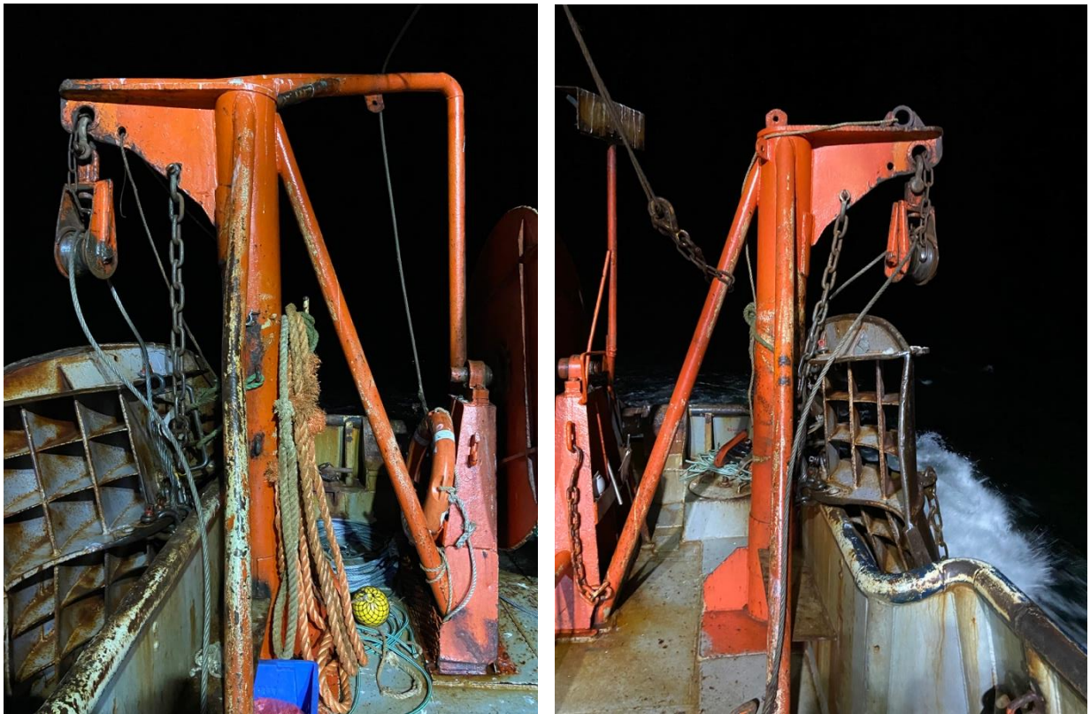
Figure 1. Stern arch system for warp cables in demersal trawl for crustaceans, at HCS, Chile. Stern view with port side bow (right) and starboard bow (left). The latter has a curved steel tube at the top (10-15 cm diameter), to facilitate the sliding of the cod-end for discharge of catch on deck.
