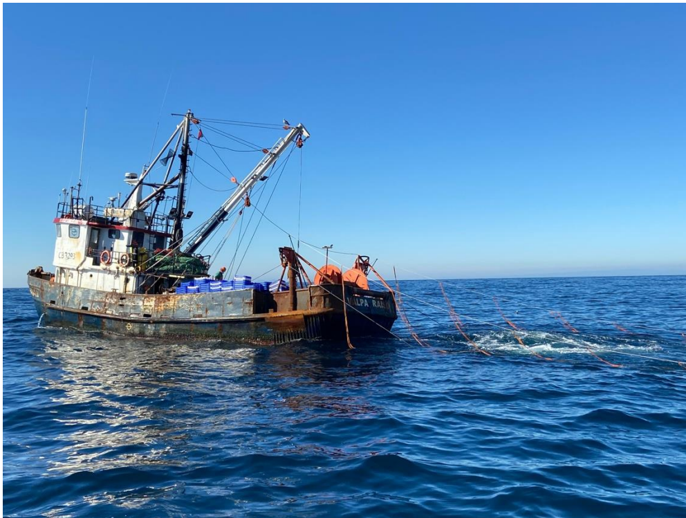
Figure 7. Bird-scaring lines deployed with extension arms onboard a small trawl vessel in the Humboldt Current, Chile.
