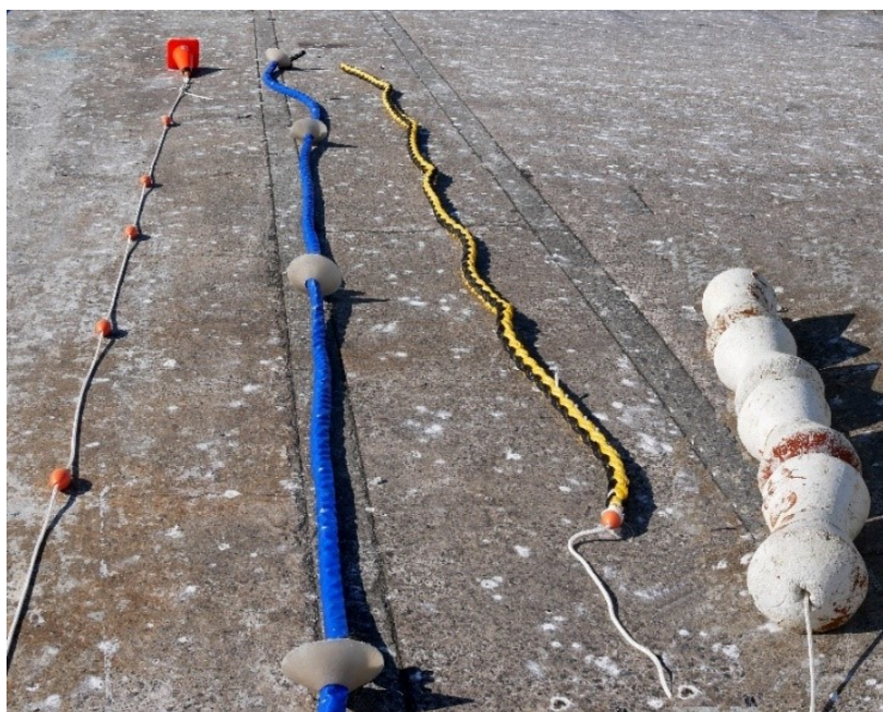
Figure 3. Photograph showing details of some of the tori line drag sections tested, from left to right: 9 mm diameter trawl braid with gillnet floats (80 mm x 45 mm) every metre and a small road cone at the end; 32 mm diameter three strand rope with fire hose and sports cones at 2 m spacing; 52 mm diameter 8 strand polypropylene rope with a 9 mm diameter trawl braid leader; Intermediate polystyrene floats (750 mm x 250 mm) on 9 mm diameter trawl braid.
