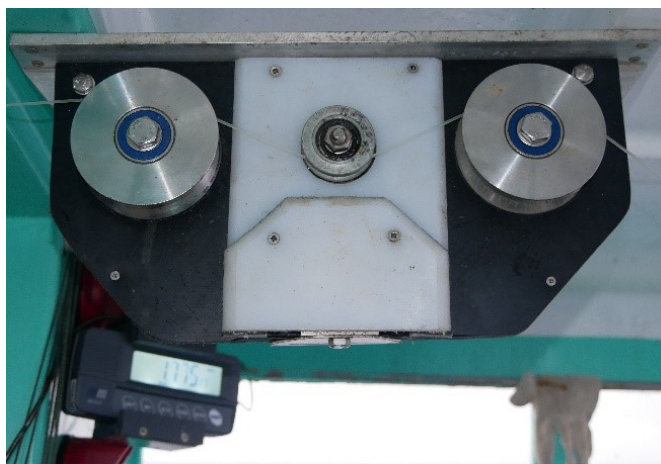
Figure 3. Photograph showing tension meter in place on the vessel, with screen in the background.
