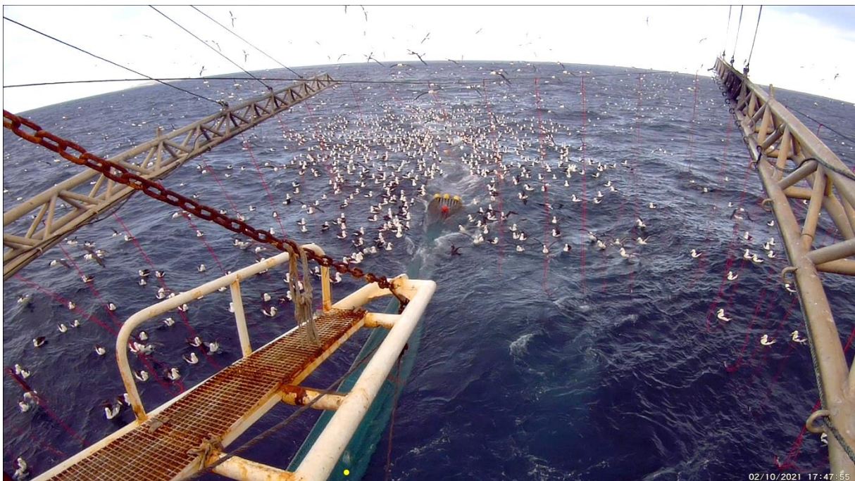
Fig.11. DIM mortality #2. The bird entered the net through the SED's top hatch (seen at the centre of the image) during the haul of station 10. The bird was originally seen alive (its position indicated by the yellow dot at the bottom of the image), however died on deck as a result of the hauling manoeuvre. The picture also shows the fixed BSL with two 15 m stern booms and three streamer curtains (two lateral, one distal), and its protected area.
