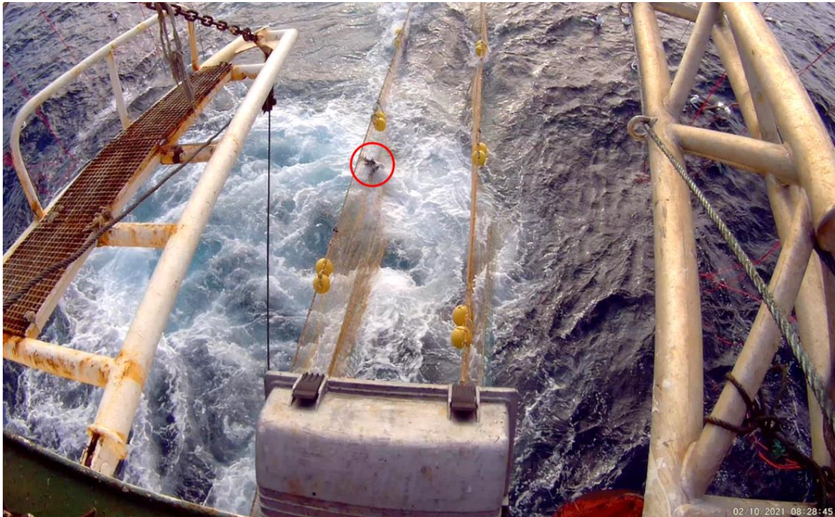
Fig.10. DIM mortality #1; carcass (indicated by red circle in image) recorded in the haul of station 6, entangled in the 200 mm mesh starboard net wing. The metal structure on the right comprises the portside boom of the fixed bird scaring lines, made of semi-flexible 10 mm red polyurethane tubing.
