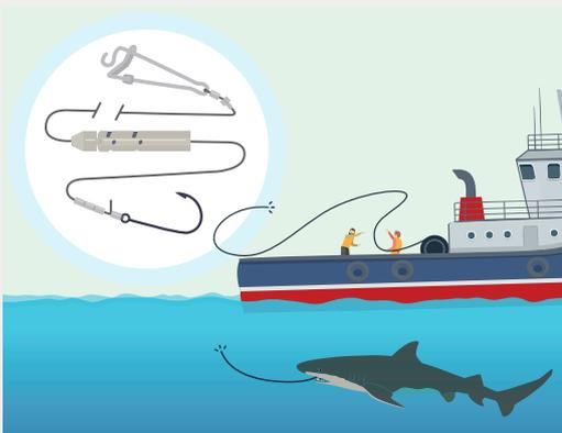
Fishermen can be injured by weights when the line suddenly breaks. Inset shows a sliding weight, a new weighting system developed to reduce the risk of injury.
