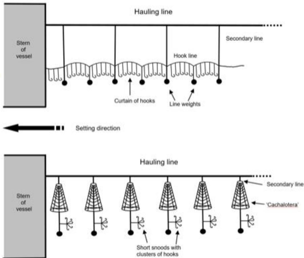
**Figure 1.** Typical configurations of the traditional Spanish double line system (a) and Chilean (trotline) system (b) showing differences in gear design and location of weights in relation to hooks. The open-ended secondary/connecting lines (not joined by a continuous hook line) and proximity of weights to hooks of the Chilean system enables hooks to sink rapidly with no lofting in propeller turbulence from the surface close to a vessel stern. Drawings not to scale.
