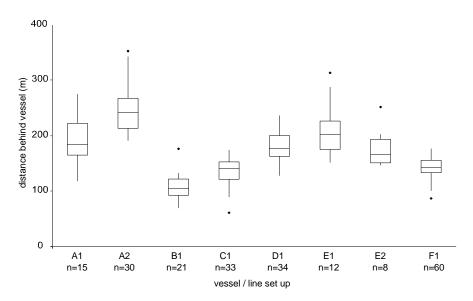
**Figure 5.** Distance behind the vessel that TDRs reached 15m depth, for 8 different line set ups tested during normal fishing operations. B1 had the most weighting (5 kg per 100 m), A2 the least (1 kg per 100 m).
