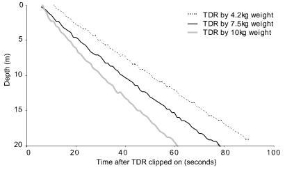
**Figure 3**. Time-depth profiles for TDRs on the same line positioned next to different sized weights
