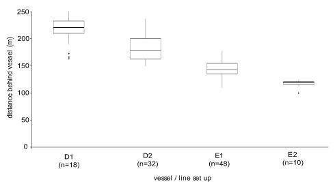
Figure 7. Distance behind vessel that TDRs reached 15 m for two different weighting regimes (1 and 2) for two vessels (D and E). Weighting regime 2 had twice as many hooks between weights as regime 1
