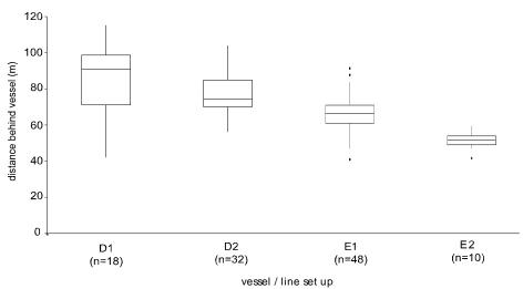
Figure 6. Distance behind vessel that TDRs reached 5 m for two different weighting regimes (1 and 2) for two vessels (D and E). Weighting regime 1 had twice as many hooks between weights as regime 2
