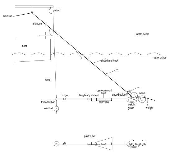
Figure 9. Prototype of underwater setting device developed by Dave Kellian.
