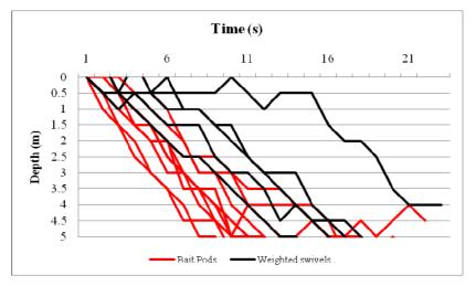
Figure 3: Sink rate profiles for bait pods and weighted swivels (60g).
