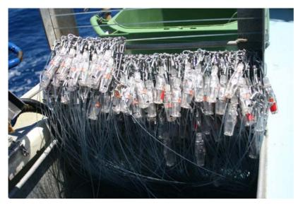
Figure 1 Hook Pods clipped onto the swive
