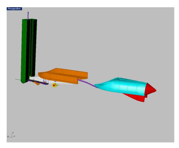
*Computer generated diagram of the bottom of the carriageway, the cradle and capsule.*
