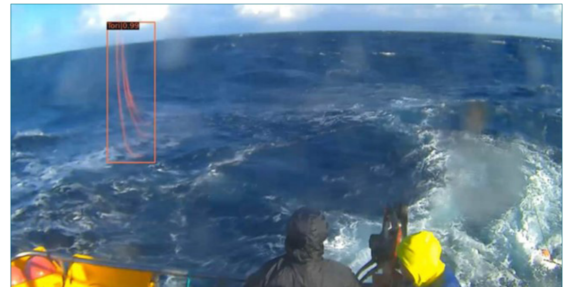
Electronic monitoring can detect if a bird scaring line is in use, but not check it meets recommended minimum specifications. Photo: CSIRO
