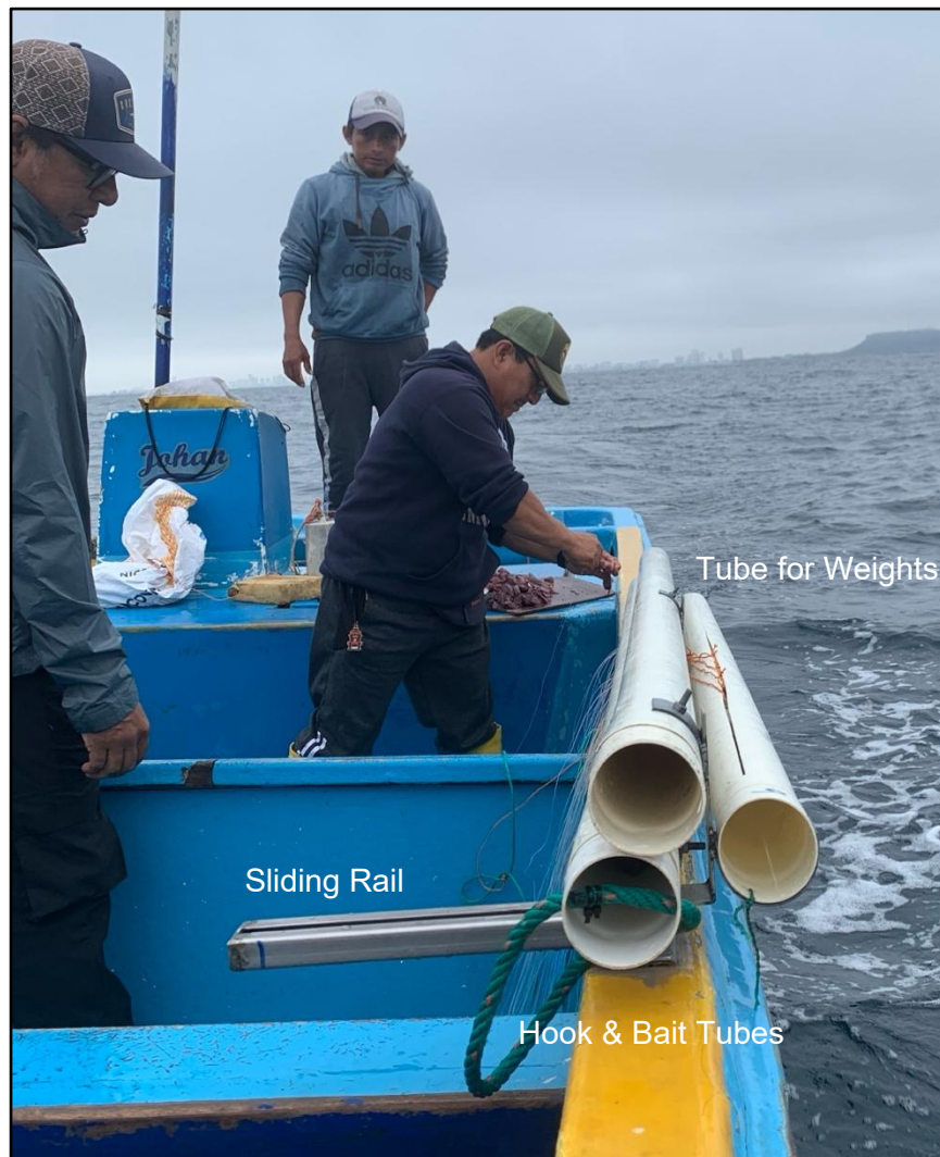
Photo 1. The 3-tube NISURI Fast-Set system installed on the gunwale of an artisanal vessel in Ecuador. Note the Sliding rail that is used to angle the system outwards from the vessel for line setting. Also note the third tube positioned to carry up to 18 concrete weights.
