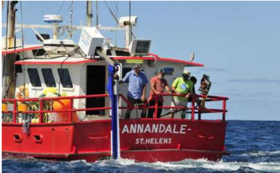
*Figure 1. The latest configuration of the MK1 underwater setting machine being trialed off eastern Australian in January 2010. The hydraulics and control box are mounted on the roof to reduce the number of pulleys involved in connecting the hydraulics motors to the capsule. Fewer pulleys increase the transfer of energy from hydraulic motors to the capsule, which increases depths attained for a given cycle time.*
