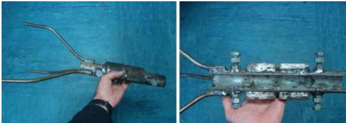
Figure 1. The corpse-catcher used to increase the likelihood of retaining seabird corpses on the warps until hauling (Photos: G. Parker).
