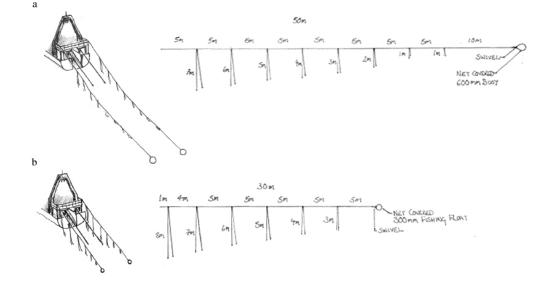
Figure 1: Schematic and dimensions of BSL designs (a) BSL-2004 and (b) BSL-2008
