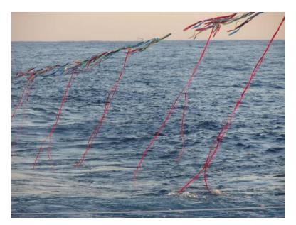
**Figure A3.** Photo of the Tori line showing the position of the long streamers (double red plastic tubes) and short coloured streamers.
