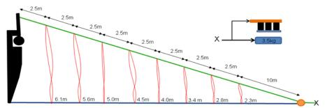
Figure 2: Tori line configuration used during experimental tests
