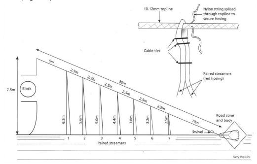
Figure 1: Tori line configuration used for experimental mitigation research
