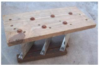
Figure 3: The towed device with 400g weights attached to the lower surface of the keels
