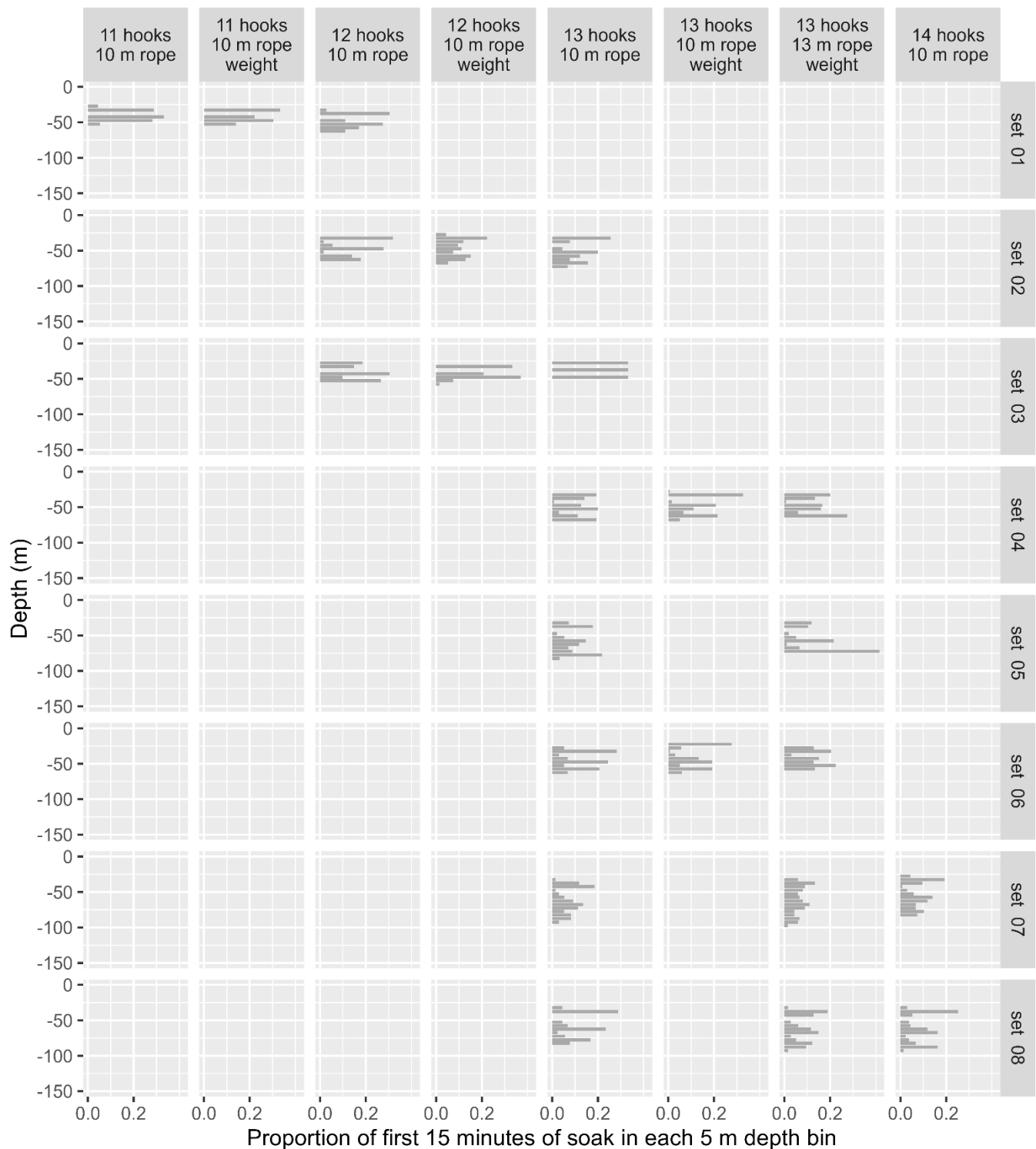
Figure A2. Histograms of TDR depth during the first 15 minutes of the soak for Trip one on Vessel A targeting bluefin tuna, by set and treatment, weight = 250-gram weight on the float rope.
