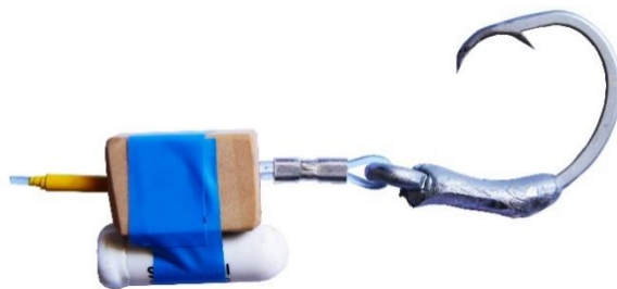
Figure 1. Time depth recorder attachment for static tests, with 16/0 50 g Procella hook, Star-Oddi DST Centi time depth recorder and float.
