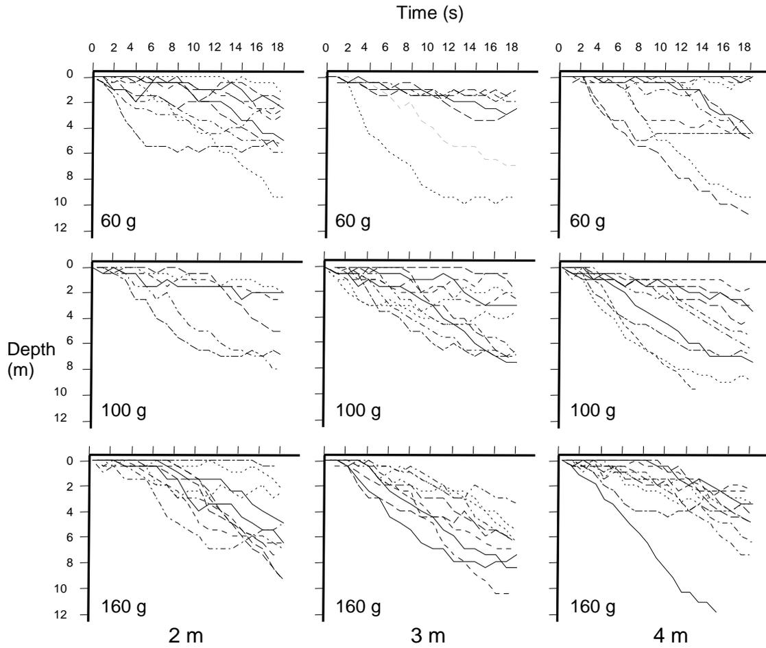
Figure 6. Sink profiles of individual live blue mackerel bait as a function of swivel weight and leader length in the first 18 seconds after deployment (corresponds to 0-6 m depth).
