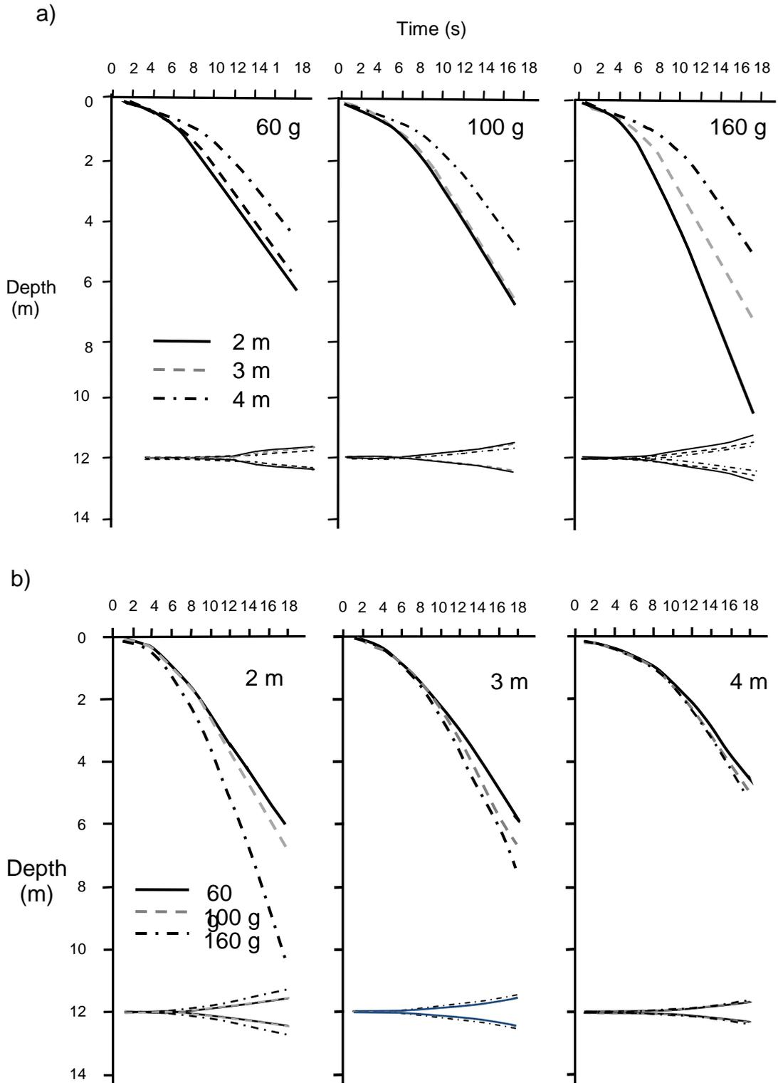
Figure 8. Mean sink profiles for the three species of dead baits (yellow-tail mackerel, blue mackerel and squid) in the first 18 seconds after deployment. The data are presented as: a) leader length as a function of swivel weight and b) swivel weight as a function of leader length. Data for the three bait species have been averaged ( $n = 33$  for each combination).
