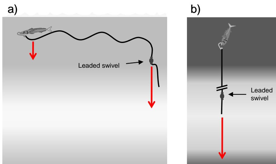
Figure 1. The source of the difference between the initial (part ‘a’) and final (part ‘b’) stages of line sinking. Landed baits sink slower than the leaded swivel until the length
