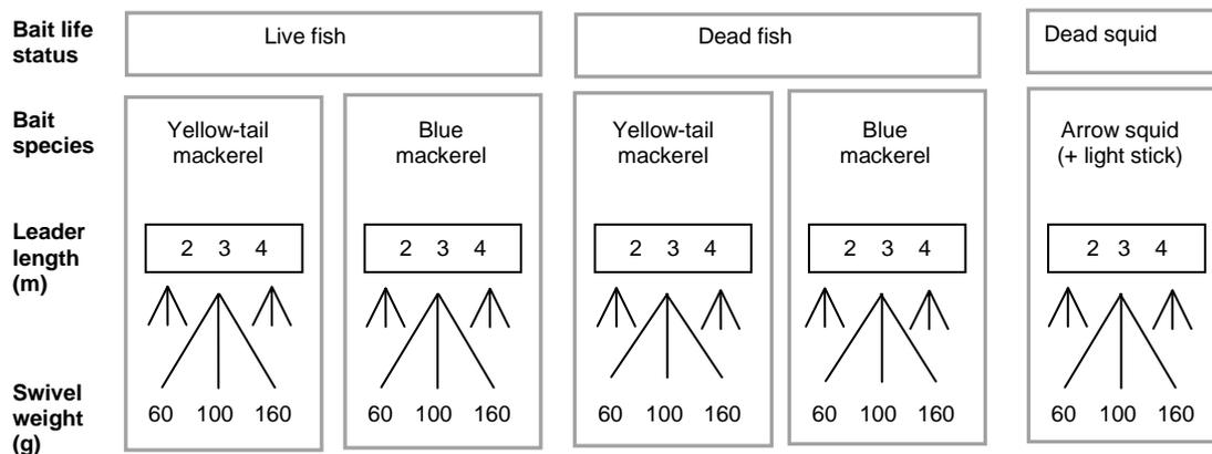
Figure 3. Experimental design showing the hierarchical order of factors testing for the effects of bait life status, bait species, leader lengths and swivel weights on the sink rates of baited hooks. The figure has been simplified for clarity. The boxes around bait species highlight the absence of live squid (no live squid used in the fishery) and the boxes encompassing the leader lengths indicate that within each of the three levels of leader lengths there were three levels of swivel weights.
