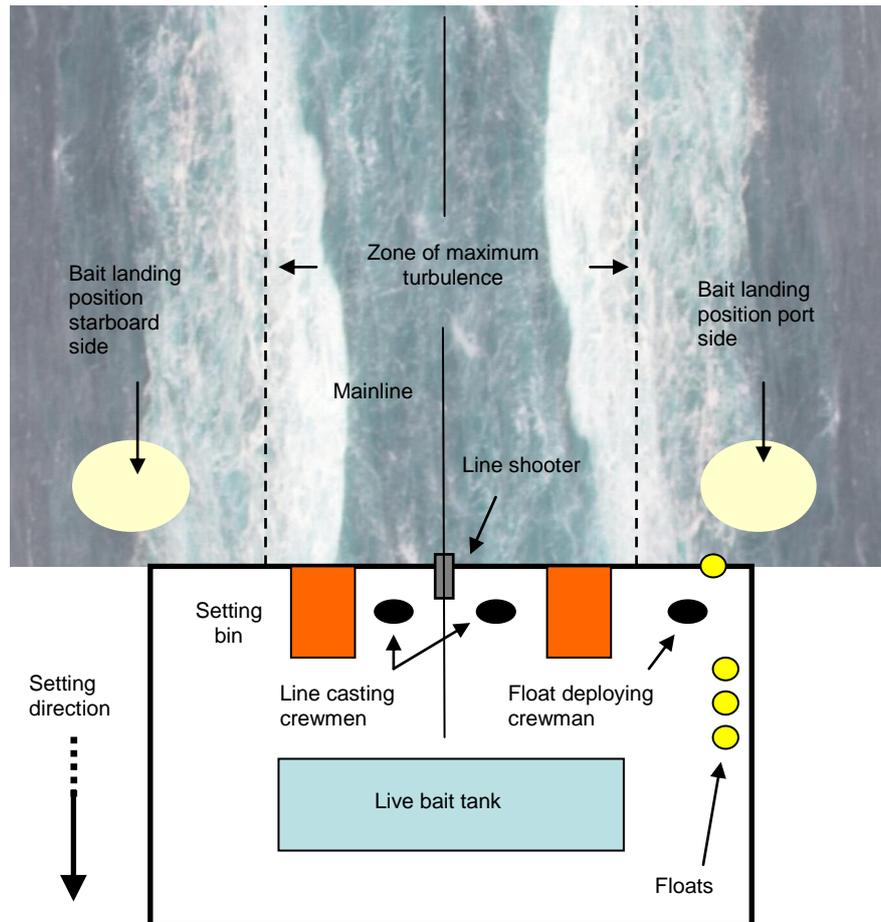
Figure 4. Line casting set-up and bait landing positions in relation to the main area affected by propeller turbulence.
