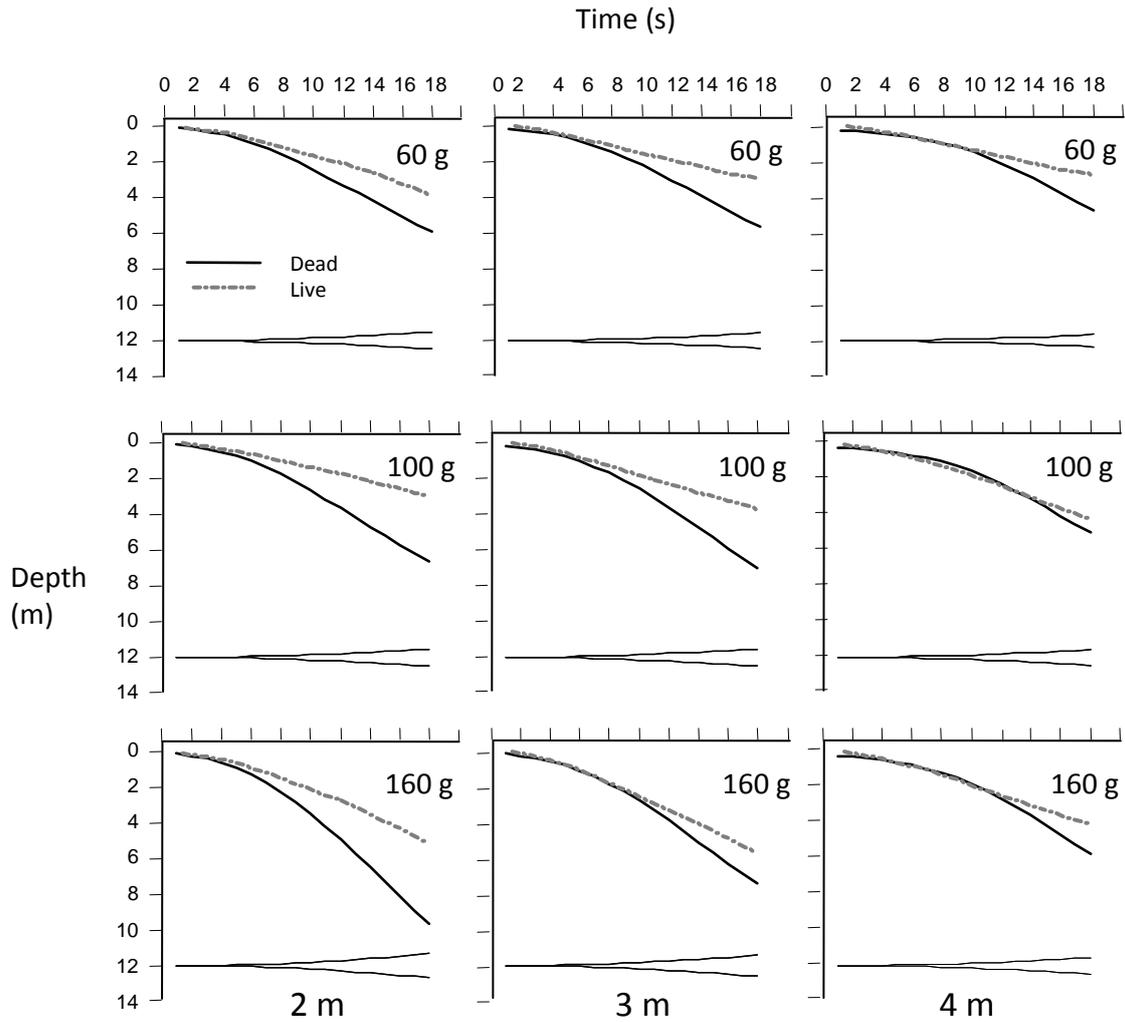
Figure 5. Mean sink profiles of dead and live yellow-tail mackerel and blue mackerel bait in relation to swivel weight and leader lengths in the first 18 seconds after deployment. Data for both fish species have been averaged (see text and Table 1).  $n = 22$  for each swivel weight  $\times$  leader length combination
