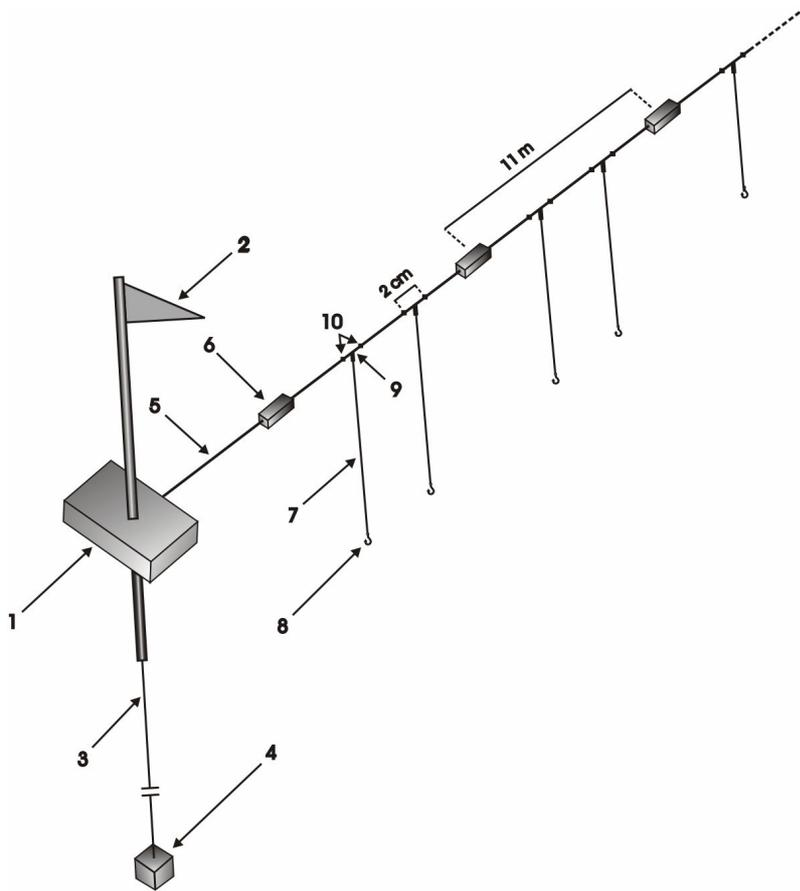
**Figure 3.** Scheme of the surface longline fishery gear targeting Dolphinfish, *Coryphaena hippurus*, in Brazilian fishing grounds. **1.** main buoy; **2.** flag; **3.** anchor line, 35 m long; **4.** stone, 3 kg; **5.** multifilament main line, 2-5 nautical miles long; **6.** secondary Styrofoam buoys; **7.** monofilament 1.4 mm secondary lines, 2 m long; **8.** 'J' hook, size 12-14; **9.** swivel, **10.** knots at the main line.
