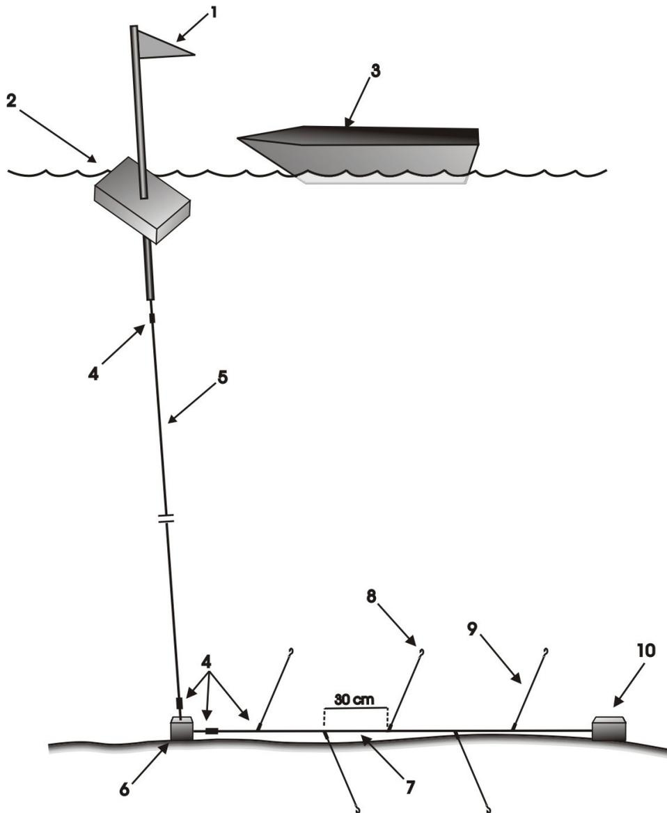
**Figure 5.** Bottom dropline gear. **1.** flag; **2.** buoy; **3.** small boat, 2 m long; **4.** swivel; **5.** main line, nylon monofilament 3.5 mm, 50 to 400 m long; **6.** weight or stone, 5 kg; **7.** main line, nylon monofilament 2.5 mm, 35 m long; **8.** hook 5 cm total length; **9.** monofilament secondary lines 1.5 mm, 0.4 m long; **10.** weight or stone (10 kg). Fishermen are unlikely to operate with both small vessels and buoy+flag, but both are shown for clarification.
