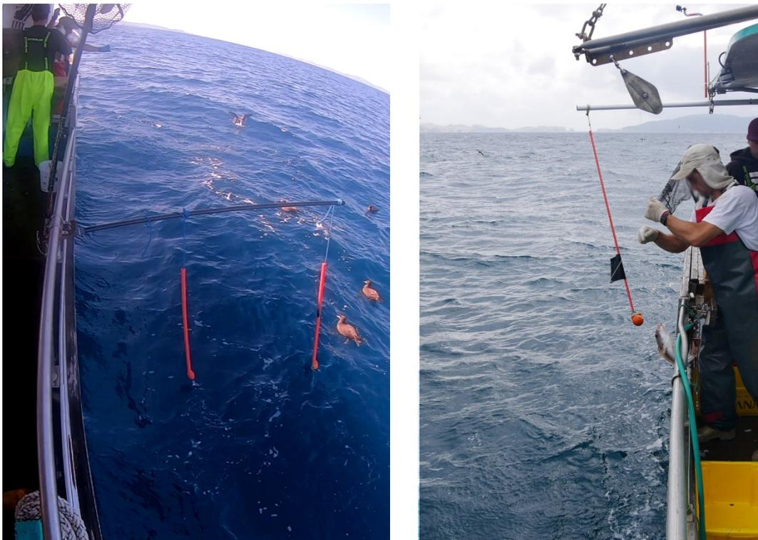
**Figure 1.** Photograph showing baffler (left, looking forwards) and dangler (right, looking aft) devices trialled on demersal longliner, vessel J. Camera position can be seen at the top right of the second photograph.
