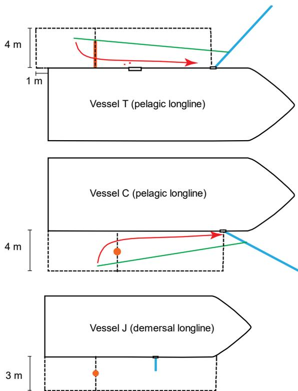
**Figure 5.** Schematic diagram showing observation boxes. The typical mainline position is shown in blue, and for pelagic longliners, the green line represents a branchline position when the hook breaks the surface, and the red line shows the path the hook takes as it is hauled by hand along the surface. The mitigation device is shown in orange, and the dotted lines represent the observation boxes.
