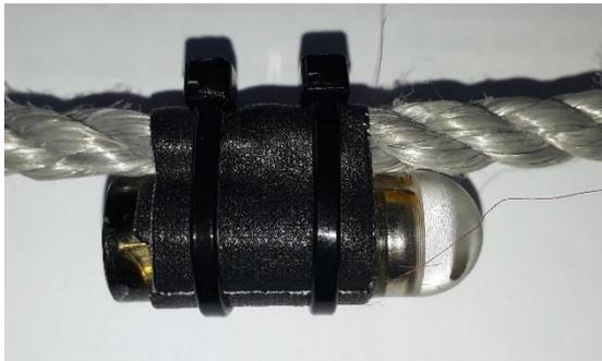
**Figure 2.** Attachment of a CEFAS G5 Time Depth Recorder to the hook line
