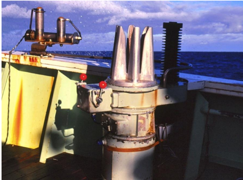
Fig 1. The bird bycatch mitigation benefit of these hydraulic branchline retrieval devices on DW pelagic longline vessels is obvious, although unsubstantiated. They allow uninterrupted fast rate of hauling, which denies birds' access to hauled hooks.
