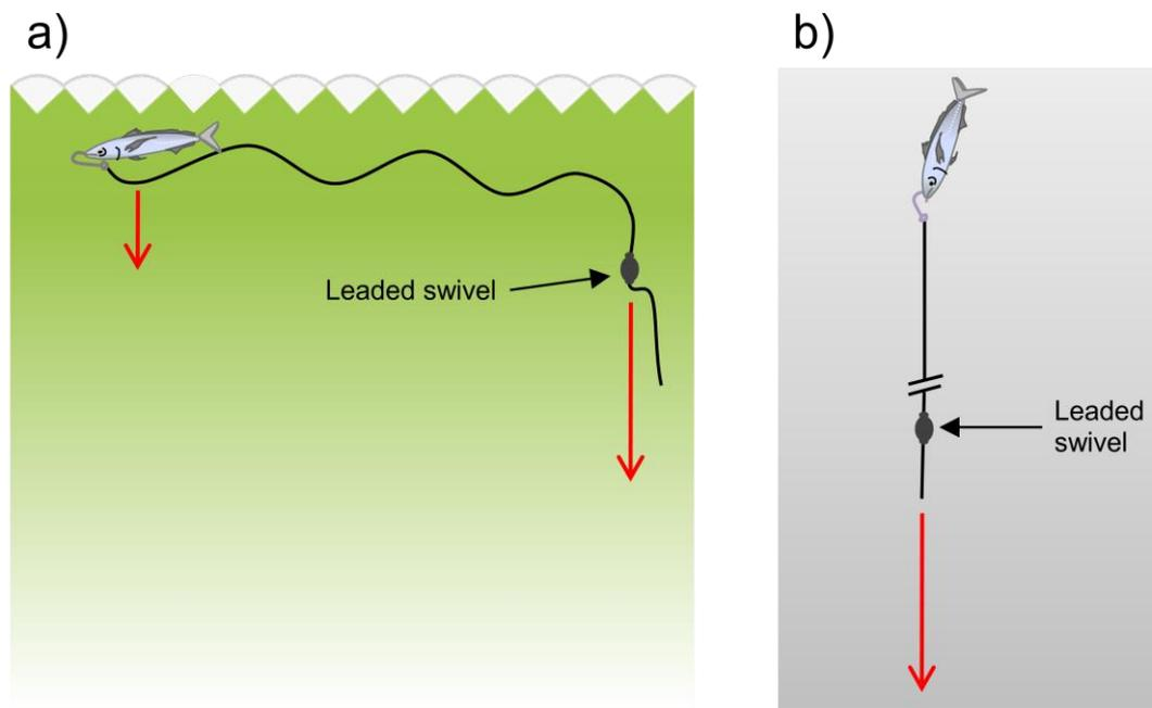
Figure 1. Sink profile of a baited hook: a baited hook sinks in two stages: (a) slowly at first until the length of line connecting the baited hook to the lead weight becomes taut, and (b) more quickly thereafter, as the lead weight engages fully on the baited hook pulling it down, resulting in a curved sink profile.
