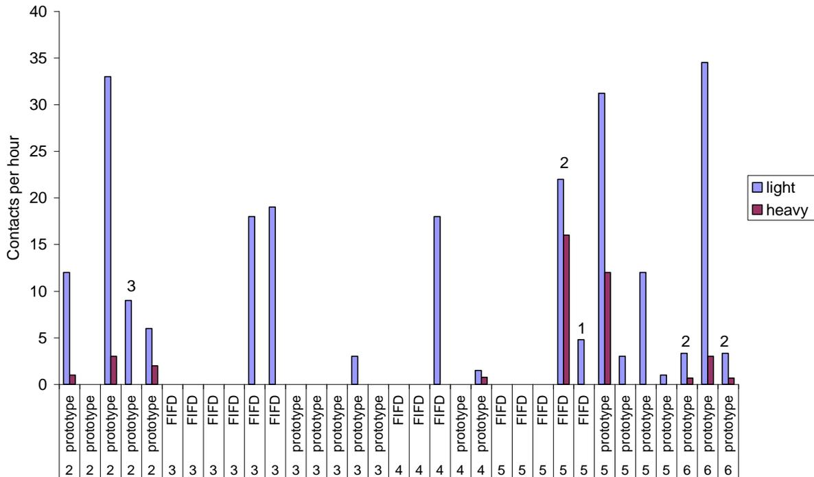
Figure 2. Contacts per hour between seabirds and trawl gear using standard FIFD BSLs (FIFD) (n=14) and experimental aerially mounted BSLs (prototype) (n=19) relative to sea state (2-6). The figures above the bars represent the number of seabird mortalities recorded from that station. Stations with no discarding occurring during the trawl are not included in this figure.
