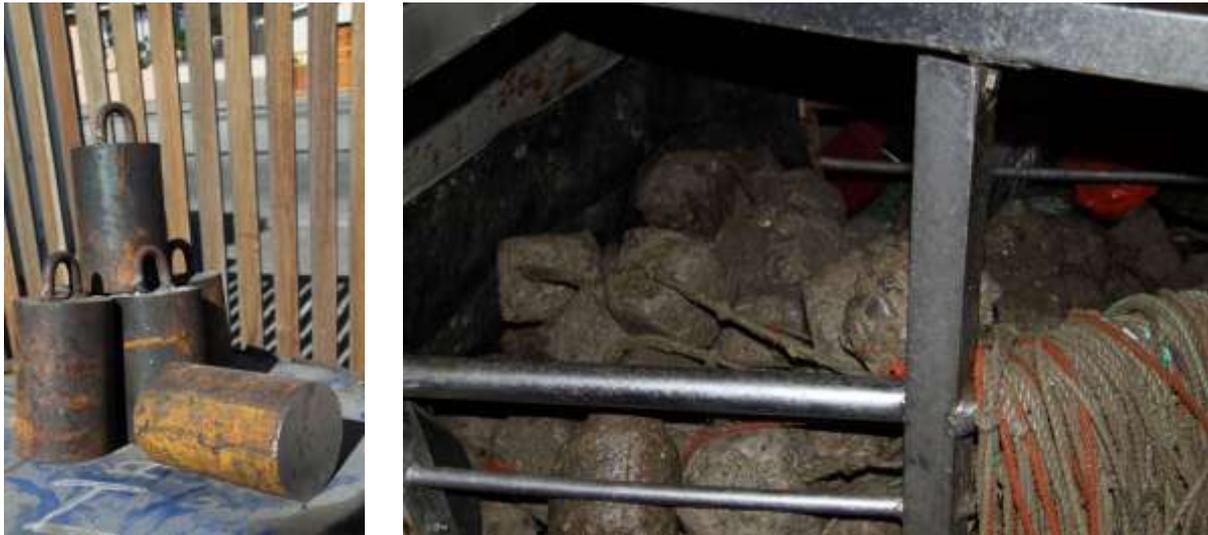
Figure 2: 5 kg steel (left) and concrete (right) weights used in experimental trials in the Namibian demersal longline fleet.
