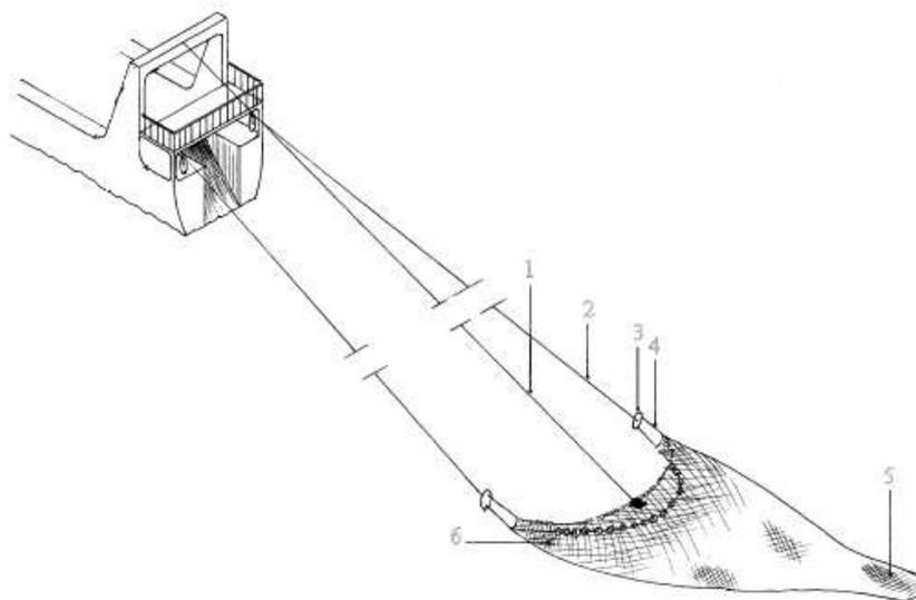
Figure 1: Working gear of a demersal trawl vessel: 1, Third wire (netsonde); 2, Warp cable; 3, Trawl door; 4, Bridle and sweep; 5, Cod end; 6, Net wings. Source: Sullivan *et al.* (2006a)
