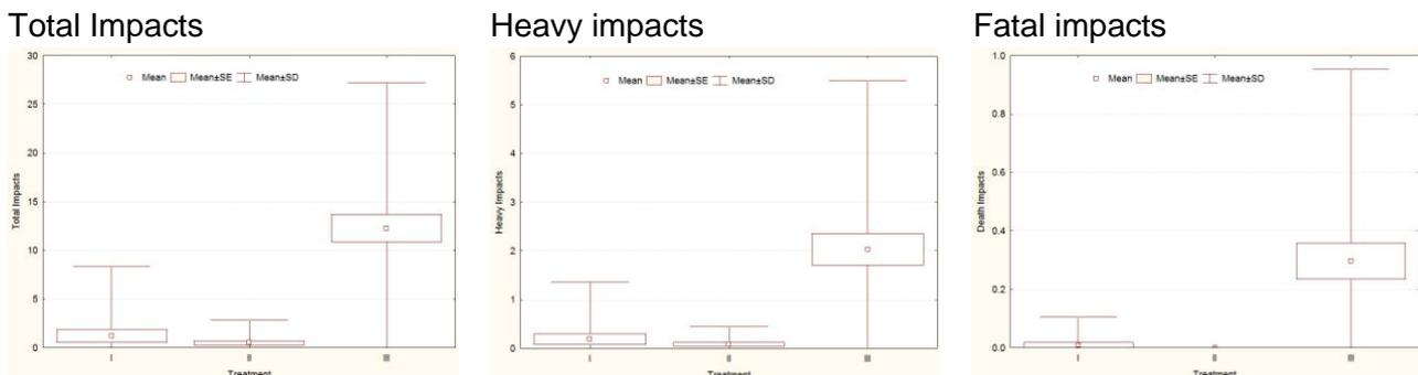
Figure 4: Total, heavy and fatal seabird impacts with warp cables recorded for each treatment. The X axis shows treatment; Treatment 1, tori line + buoy (left); Treatment 2, tori line + off-setting towed device (middle); and Treatment 3, control (right).
