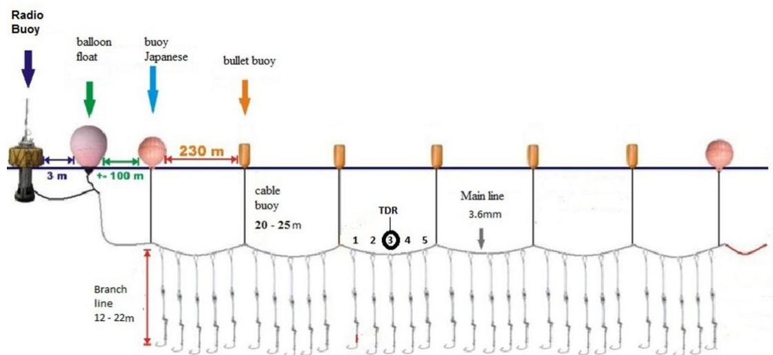
Figure 2: Basic configuration of Brazilian pelagic longline gear, showing the position where TDRs were attached in relation to hooks between buoys.
