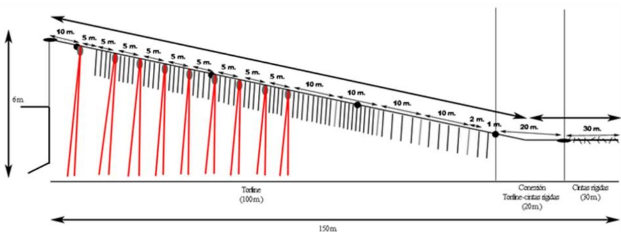
Figure 7: Schematic of the tori line design used in Uruguayan pelagic longline vessels throughout the experiment.
