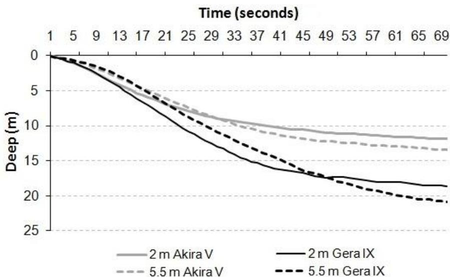
Figure 3: Mean sink profiles of baited hooks for Treatment 1 (2 m) and 2 (5.5 m), from data collected on FV *Akira V* (Treatment 1:  $n = 44$ ; Treatment 2:  $n = 45$ ) and FV *Gera IX* (Treatment 1:  $n = 15$ ; Treatment 2:  $n = 13$ ).
