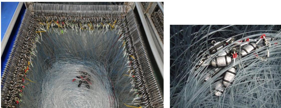
Figure 1. Snood bin of the Samurai as used in the 120 g at 2 m trial (left). Clips (one end of the branch line) are attached to horizontal runners around the top of the bin and hooks (the other end of branch lines) are suspended from the clips. The branch lines are coiled in the bin along with the line weights. Some branch lines shown are fitted with sleeves adjacent to the hooks. The yellow cable ties shown were attached for experimental purposes and are not
