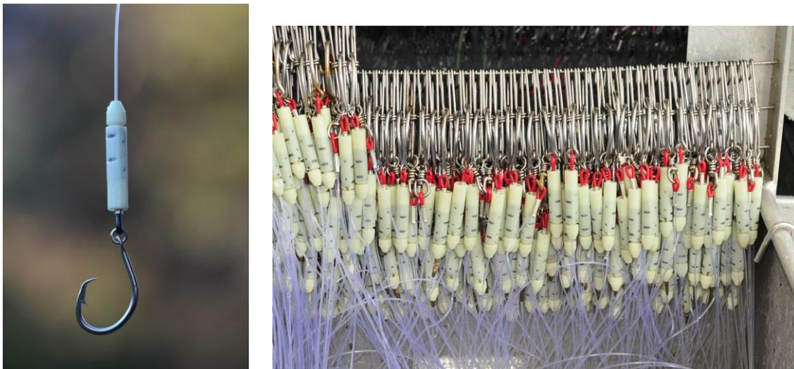
Figure 2. A 40 g Lumo hook lead and a # 14/0 circle hook (left). The lower on-third of the lead is rebated to fit over the crimp. The photo on the right shows 40 g Lumo leads stitched into the branch lines in a gear bin.
