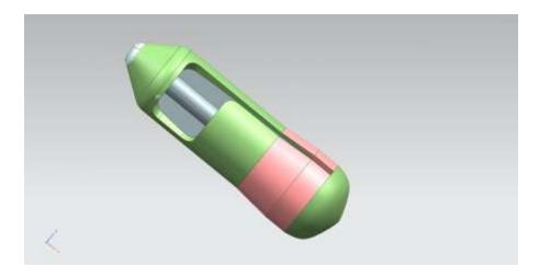
Figure 3. Latest design of the bait holding capsule (differs from that shown in Figure 1). Following extensive computer modeling and at-sea testing, this design incorporates twin (opposing) bait chambers and refines the orientation between the centre of gravity and the centre of buoyancy. The latter is considered critical to maximizing depths attained and minimizing the time between deployments.
