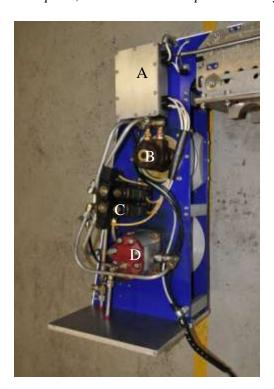
Figure 2. The drive system of the underwater setter. Shown are the control box (houses the PLC, data recorder and GPS; A), recovery motor (B), solenoid and relays (C) and pull-down motor (D). The on/off button and brake and timer are on the other side. The pulleys holding the spectra rope are barely visible beneath the hydraulic motors.
