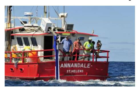
Figure 1. The latest configuration of the MK1 underwater setting machine being trialed off eastern Australian in January 2010. The hydraulics and control box are mounted on the roof to reduce the number of pulleys involved in connecting the hydraulics motors to the capsule. Fewer pulleys increase the transfer of energy from hydraulic motors to the capsule, which increases depths attained for a given cycle time.
