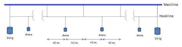
Figure 1: Namibian demersal longline gear configuration
