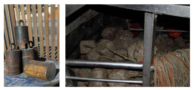
Figure 2: 5 kg steel (left) and concrete (right) weights used in experimental trials in the Namibian demersal longline fleet.
