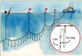
Figure 1. Pelagic longline gear configuration with line weighting. Note the distance between the weight and the hook.
