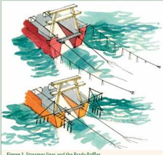
Figure 1. Streamer lines and the Brady Baffler.
