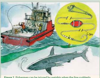
Figure 2. Fishermen can be injured by weights when the line suddenly breaks. Inset, shows the *Safe Lead*, a new weighting system being developed to reduce the risk of injury.
