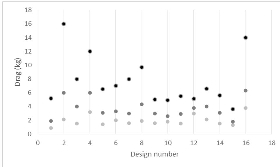
Figure 9. Drag generated from an in-water section of rope with various objects attached, at approximately 2.6 knots (light grey), 4.2 knots (dark grey dots) and 6.5 knots (black dots). Configurations of the in-water section are described in Table 2.
