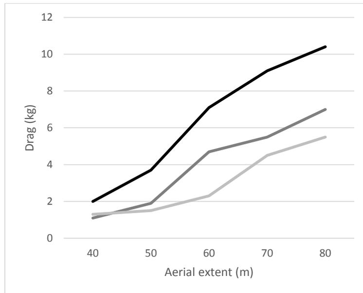
Figure 5. Drag required to achieve tori line aerial extents of 40 m – 80 m at deployment heights of 5 m (black), 7 m (dark grey) and 9 m (light grey), when 3 mm Dyneema backbone was used with streamers placed every 5 m along the line.
