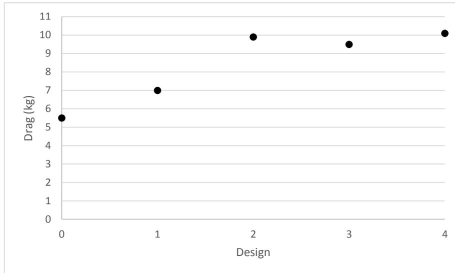
Figure 8. Drag required to provide 70 m aerial extent for a tori line with a 3 mm Dyneema backbone deployed at 7 m high, with different combinations of streamers and shark clips attached. Design 0: streamers at 5 m intervals; 1: streamers at 5 m intervals and 10 shark clips attached; 2: streamers at 2.5 m intervals with no shark clips; 3: streamers at 2.5 m with 10 shark clips; 4: streamers at 2.5 m with 17 shark clips.
