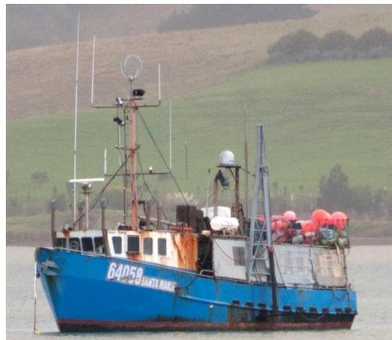
Figure 4. A vessel that fishes using both the bottom and surface longline methods, with metal shelter deck supports and a float cage near the stern. Photo: D. Goad.
