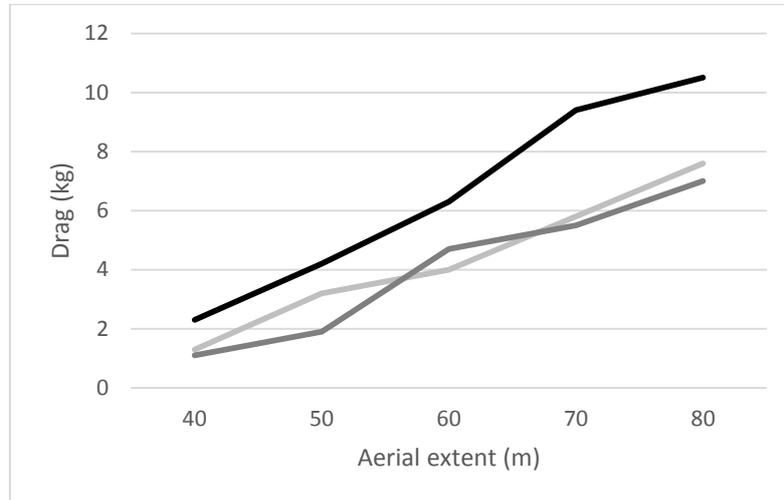
Figure 7. Drag required to achieve tori line aerial extents of 40 m – 80 m using three different backbone materials: monofilament (black), Dyneema (dark grey), Ashaway albacore braid (light grey) at a deployment height of 7 m.
