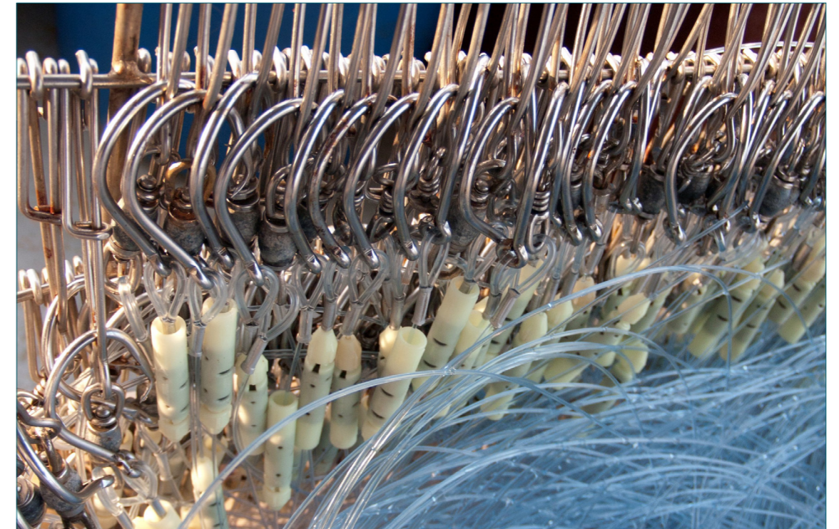
Fast sinking hooks with added weights help avoid catching seabirds.
